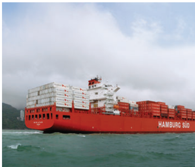
The Rio de la Plata, with a slot capacity of 5,900 TEU, is one of Hamburg Süd's largest and newest vessels. Ships in its class have 1,365 reefer container plugs.
