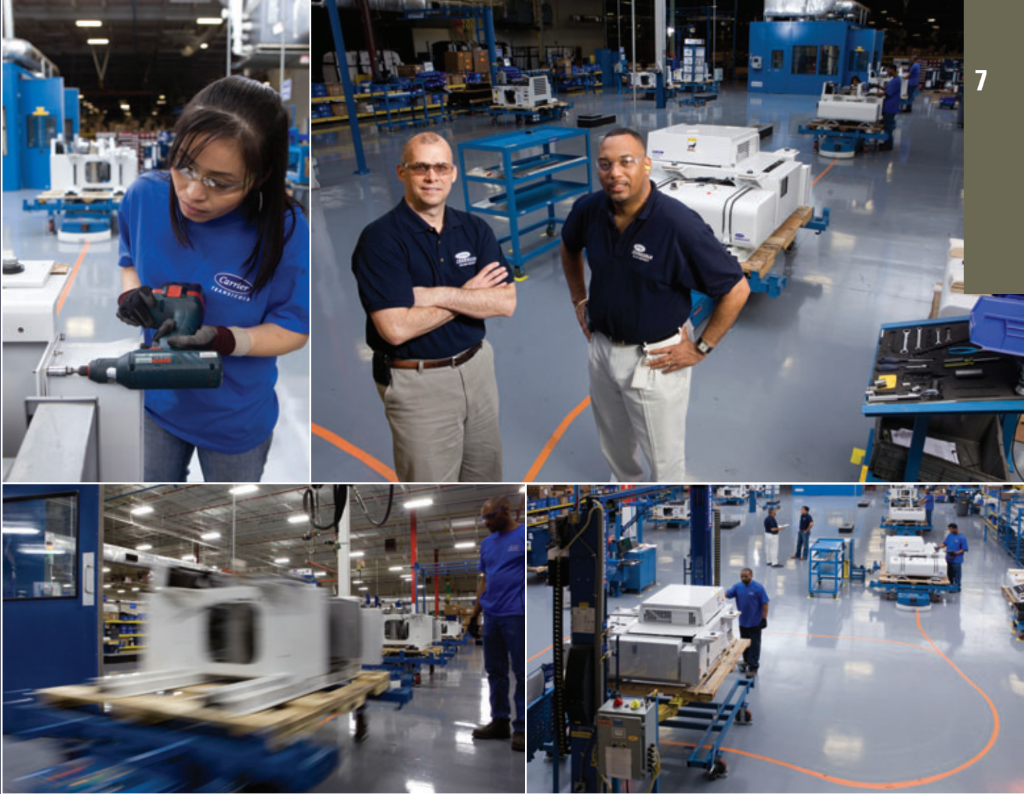
Technologies Advancing Assembly (clockwise from upper left) – Automated tools know exactly how much torque to apply to a bolt. Troy Rector, plant manager, and Geoffrey Mack, business unit manager, at the Athens plant where PowerLINE generator sets are now made. Orange lines on the floor guide automated carts to workstations. A cart scoots out of a test booth after automatically activating doors.
