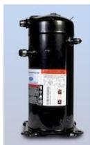
The new Vector models are also the first North American trailer units to use a fully hermetic electric scroll compressor. Proven efficient and reliable in Carrier Transicold refrigerated marine container systems, the scroll compressor has 70 percent fewer moving parts and is 200 pounds lighter than a traditional reciprocating compressor, contributing to the host unit’s overall 10 percent weight reduction compared to its predecessor.
