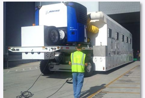
As the saying goes, failure is not an option in space missions. For that reason, Boeing requires redundant refrigeration units for its satellite transporter. The Vector 8500 units (blue) share a common supply/return plenum (white area with Boeing logo). The white ductwork carries supply air, which flows down both sides to the far end of the transporter.
