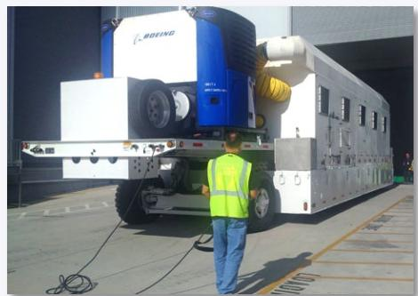
As the saying goes, failure is not an option in space missions. For that reason, Boeing requires redundant refrigeration units for its satellite transporter. The Vector 8500 units (blue) share a common supply/return plenum (white area with Boeing logo). The white ductwork carries supply air, which flows down both sides to the far end of the transporter.
