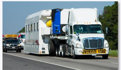
The six-day trip a Boeing satellite makes from California to the Florida launch pad requires a convoy, including chase-cars and highway patrol escorts. The Vector must run around-the-clock for each day of the trip.
