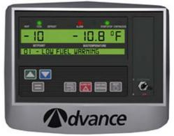
If the fuel level drops below 15 per cent for more than 30 seconds, the refrigeration unit's LED light bar glows a cautionary yellow to
