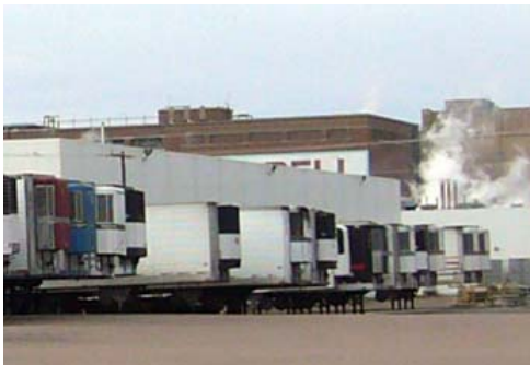
Trailers used for temporary stationary cold storage may be equipped with old refrigeration units with unregulated diesel engines that are less fuel efficient and emit more pollutants.
