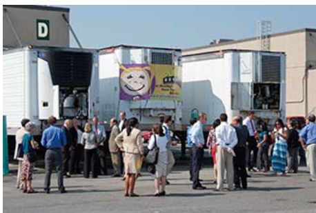
To help address serious air quality issues in Chelsea, Mass., the EPA awarded $1.9 million to the Chelsea Collaborative for diesel emission reduction technologies, including 79 all-electric Vector 5100 units from Carrier Transcold that will replace older diesel engine powered units at the New England Produce Center, the nation's largest produce market. The open Vector unit is on the left.
