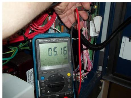
If 5.2 VDC is not present, check wiring between controller and the module, and retest.
