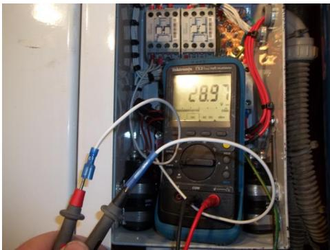
If voltage is not present, repair power supply. If voltage is present, proceed to testing the scrubber motor output.
