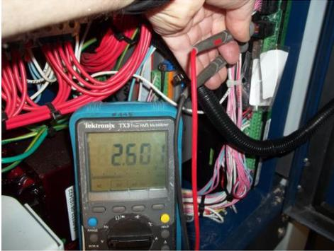
If voltage at MC1 does not change, verify the input voltage to the GIM module by opening the XF control box and checking voltage between XST1 (+) and XC1 (-). When scrubber is operating in “tEst” mode, the voltage should be between 17.2 VDC and 30 VDC.
