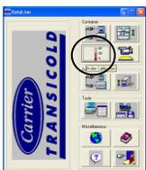
If the reading is greater than 0.2 °C from 0 °C, recalibration of the probes is required. Connect laptop to unit and start DataLine. From the Launch Pad screen, select the probe calibration button (2<sup>nd</sup> button on the left). Ensure the connection between the laptop and the unit is good. In the probe calibration screen, the values will show x if the connection is not good.
