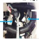
schrader fitting during the install. It is recommended that after you reinstall the fitting that you leak check the connection.
