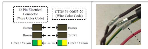
5. Perform the following 3, two-to-one butt splice electrical connections as shown.
