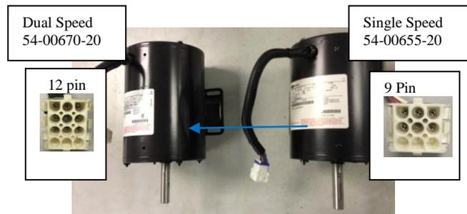
1. From a failed CM (54-00670-20), cut the wires (150mm or 6”, measured from the 12 pin connector end) using a wire cutter and strip off (5mm or 0.2”) the wire insulation using a wire insulation stripper.
