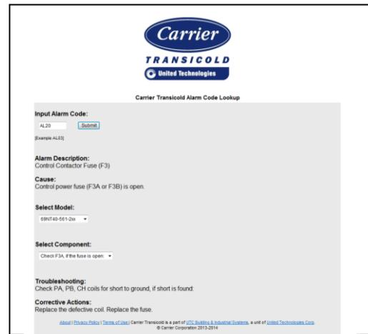
The application provides the basic alarm description, potential causes and repair actions. This simplifies troubleshooting and, in turn, saves technicians time by not having to find and refer to the manual.
