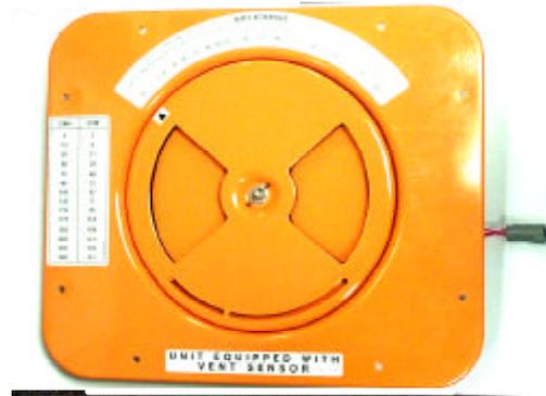
The vent position will display for 30 seconds whenever motion corresponding to 5 CMH (3 CFM) or greater is detected. It will scroll in intervals of 5 CMH (3 CFM).
