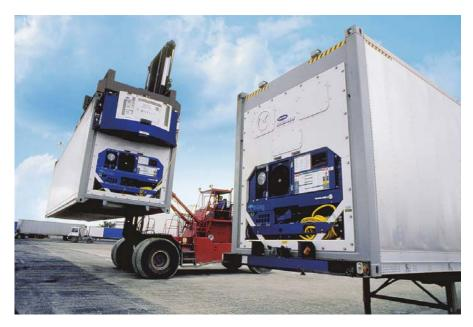
The PowerLINE® clip-on generator set (shown) and PowerLINE undermount generator set can get, under certain circumstances, up to a 25 percent boost to fuel efficiency with a new dual-speed option.
