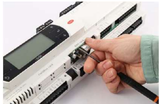
Figure 2.e - Removal of pCOWeb from controller
