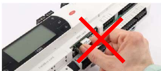
Figure 2.f - Do not pull up pCOWeb using the Ethernet connector
