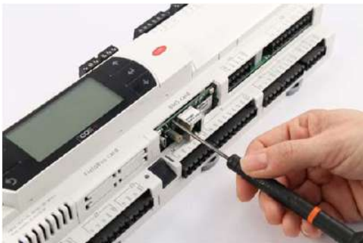
Figure 2.e - Removal of pCOWeb from controller
