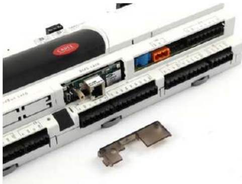
Figure 2.c - Inserting pCOWeb in the pCO controller
