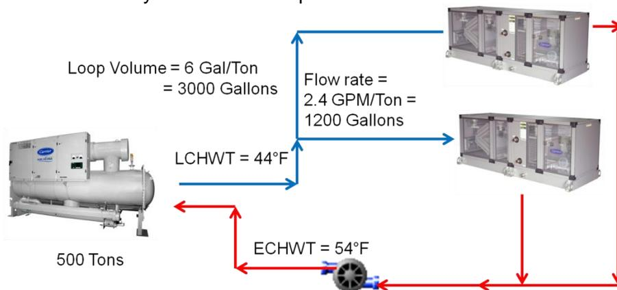
Figure 3 - Large Loop Volume System during Transient
