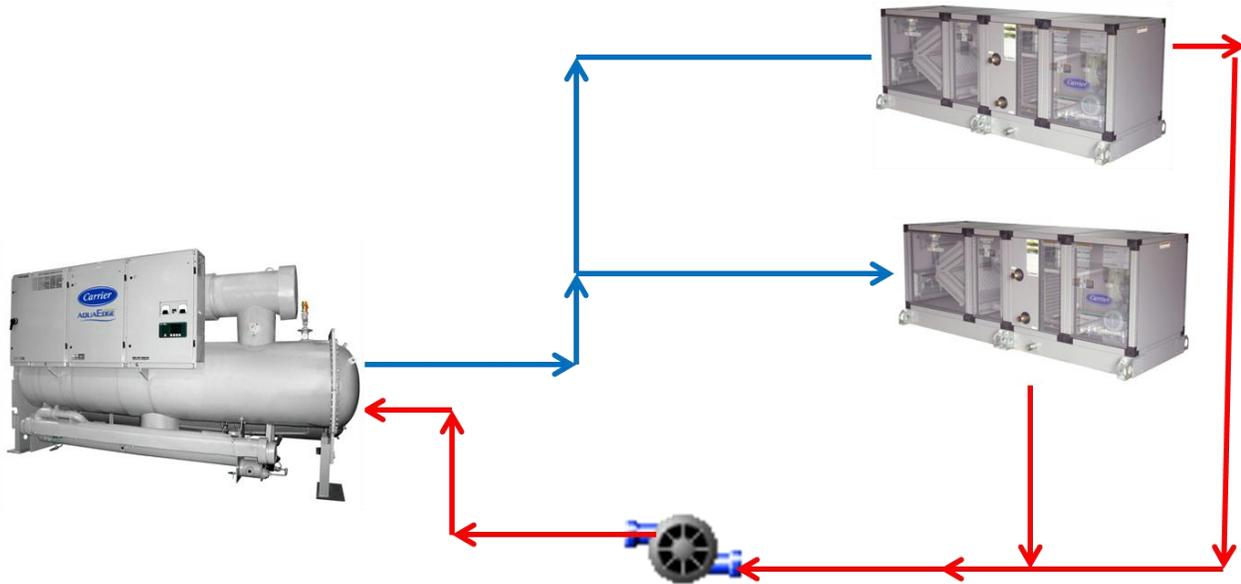
Figure 2- Simple Chilled Water Loop
