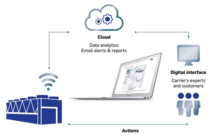
Carrier connected services allows you to track and monitor your HVAC equipment systems performance and operating parameters in real time. This allows the user to perform any required preventative and corrective actions remotely, as well as have the full analysis of your chillers at your fingertips regardless of your location.
