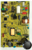
MCC-1626 : Control, LED check code, miss-wiring protection circuit.
