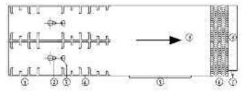
Horizontal cross section of infrasonic humidifierer
