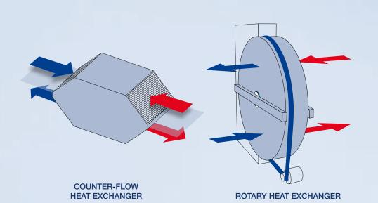
adapted to environments where flows of fresh and extracted air must be airtight. A **rotary heat exchanger** provides optimal heat
