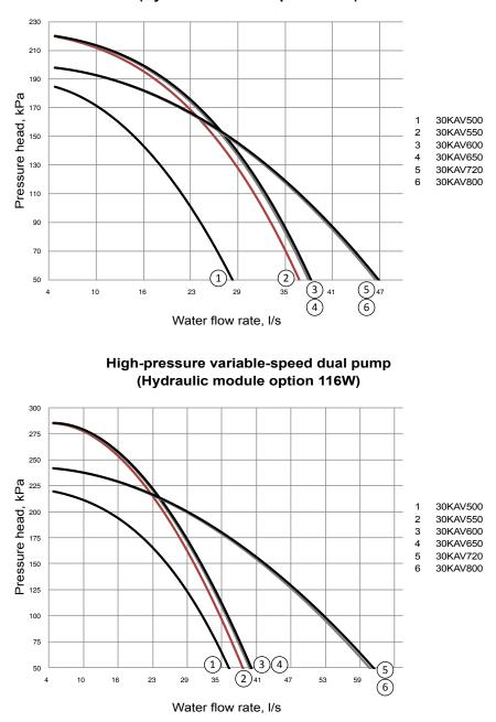
Low-pressure variable-speed dual pump (Hydraulic module option 116A)
