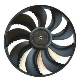
The 30KAV utilizes Carrier's the 6th generation Flying BirdTM fan technology, engineered for maximum efficiency, super low noise, and wide operating range. The fan includes Carrier patented rotating shroud technology and back-swept blades with a unique wave-serration trailing edge inspired from nature.
