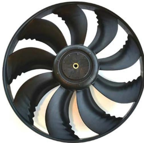
The 30XB and 30XBP utilize Carrier’s 6<sup>th</sup> generation Flying Bird™ fan technology, engineered for maximum efficiency, super low noise, and wide operating range. The fan includes Carrier patented rotating shroud technology and back-swept blades with a unique wave-serration trailing edge inspired from nature.
