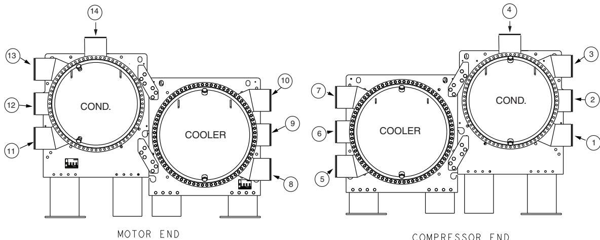
**19XR TWO-STAGE COMPRESSORS FRAME SIZES 6 AND 7 FRAMES A, B, C, AND D
