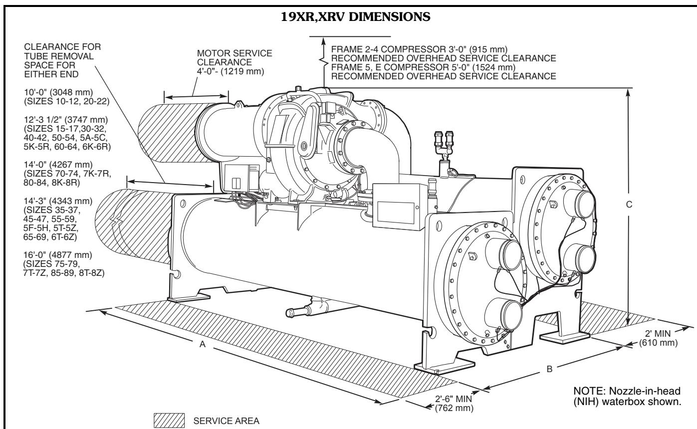
**19XR,XRV DIMENSIONS — SINGLE-STAGE COMPRESSOR AND TWO-STAGE COMPRESSOR FRAME SIZE E
