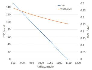
Airflow performances curve with factory installed filters (MERV 7 and HEPA H13), 230V, without duct.
