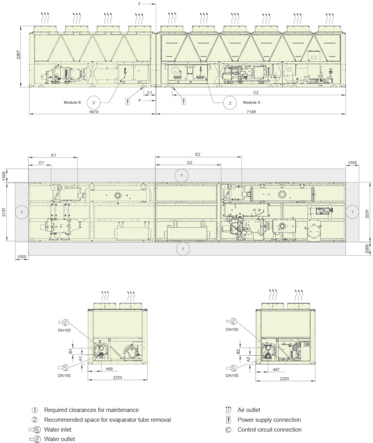
Notes: Drawing for 30XQ1150-1230 Double power connection point, and arrive from the bottom. Reserve 120mm height space below the unit for power supply connection (unit aerial installation or cable slot arrangement in unit base). Two water connection piping should be prepared.
