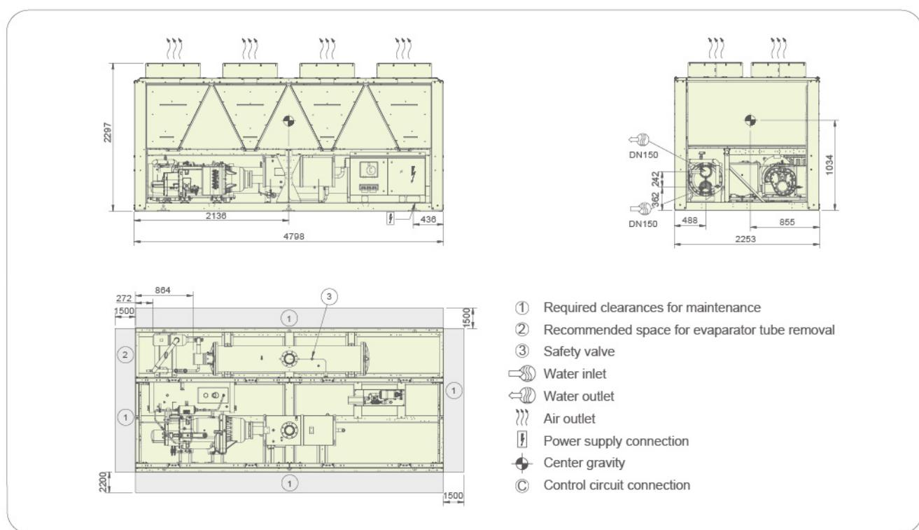
Notes: Single power connection point, and arrive from the bottom. Reserve 120mm height space below the unit for power supply connection (unit aerial installation or cable slot arrangement inunit base)
