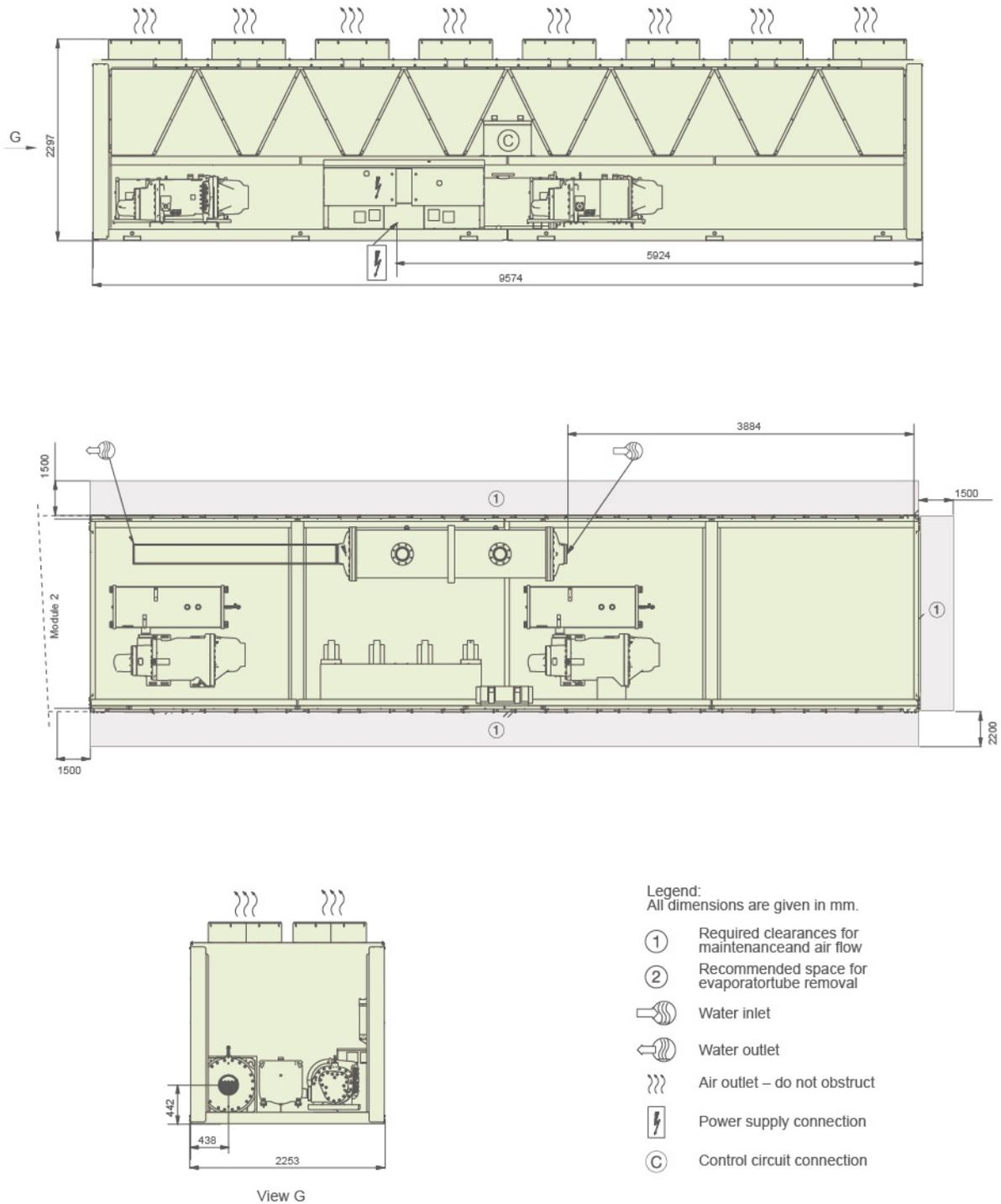
Note: Dual point power connection (Single point power connection as option), power cable arrive from bottom of electrical box, reserve at least 120mm height space below unit for power supply connection (unit aerial installation or cable slot)
