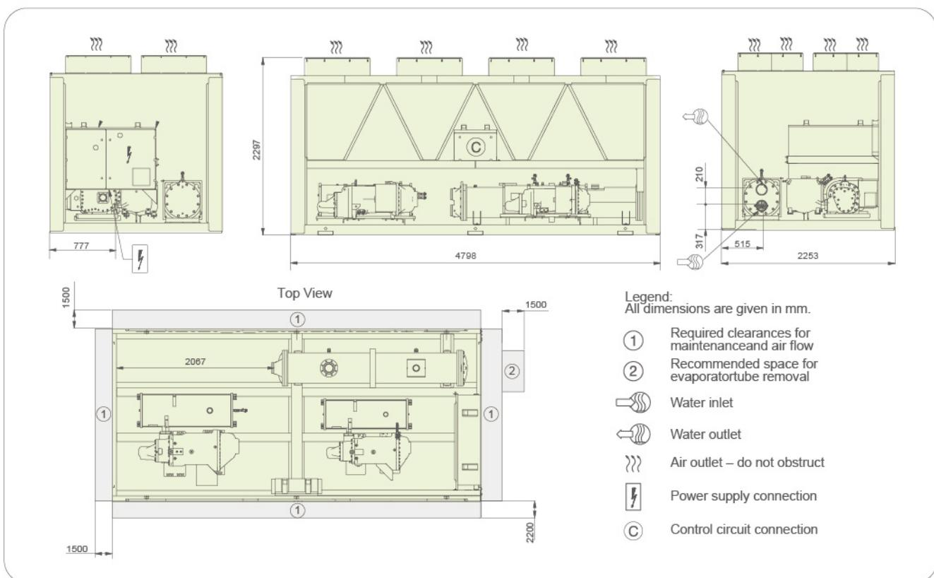
Note: Single point power connection, power cable arrive from bottom of electrical box
