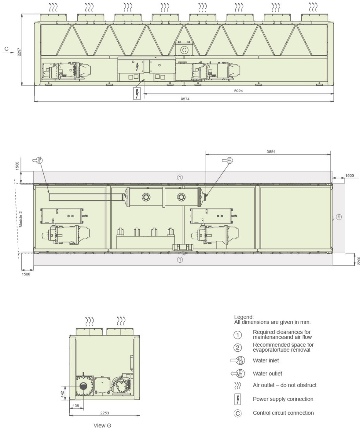
Note: Dual point power connection (Single point power connection as option), power cable arrive from bottom of electrical box, reserve at least 120mm height space below unit for power supply connection (unit aerial installation or cable slot)
