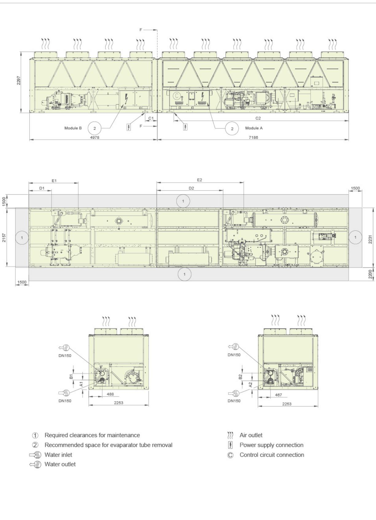
Notes: Drawing for 30XQ1150-1230 Double power connection point, and arrive from the bottom. Reserve 120mm height space below the unit for power supply connection (unit aerial installation or cable slot arrangement in unit base). Two water connection piping should be prepared.
