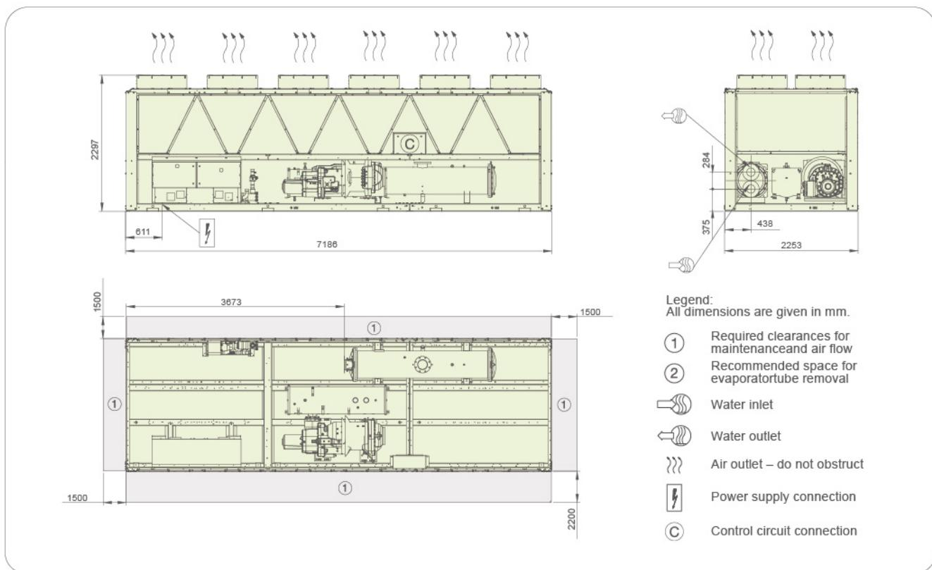
Note: Single point power connection, power cable arrive from bottom of electrical box, reserve at least 120mm height space below unit for 30XA0652~0762 power supply connection (unit aerial installation or cable slot)
