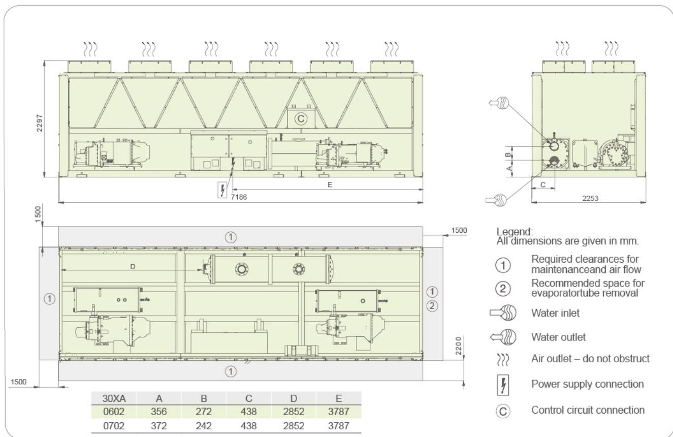
Note: Single point power connection, power cable arrive from bottom of electrical box, reserve at least 120mm height space below unit for 30XA0602~0702 power supply connection (unit aerial installation or cable slot)
