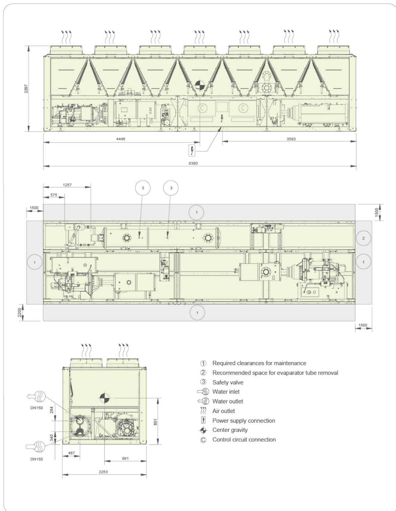
Notes: Single power connection point, and arrive from the bottom. Reserve 120mm height space below the unit for power supply connection (unit aerial installation or cable slot arrangement in unit base)
