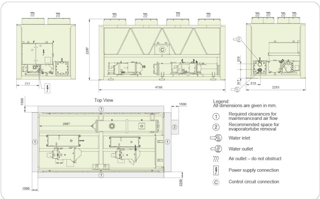
Note: Single point power connection, power cable arrive from bottom of electrical box
