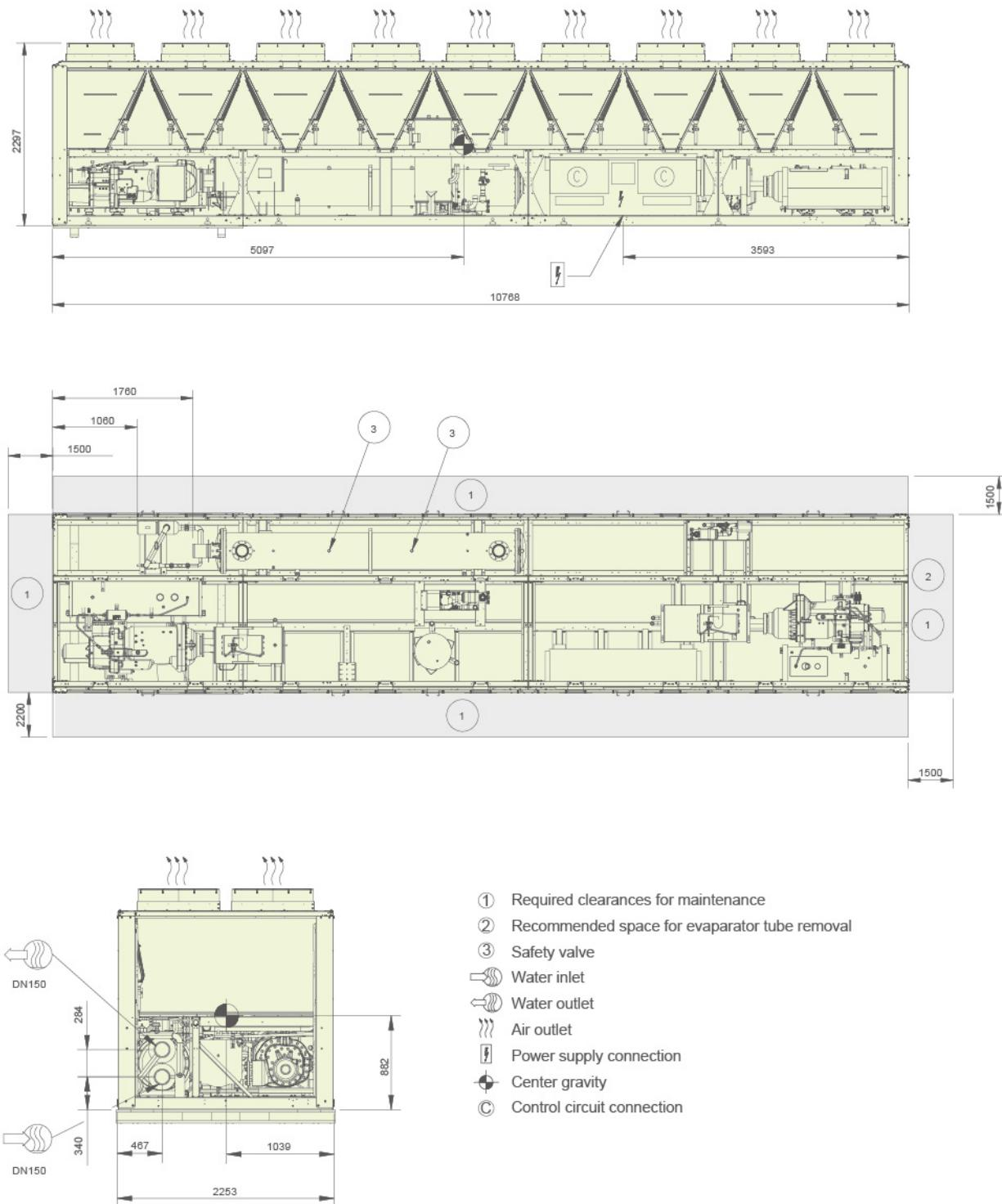
Notes: Single power connection point, and arrive from the bottom. Reserve 120mm height space below the unit for power supply connection (unit aerial installation or cable slot arrangement in unit base)
