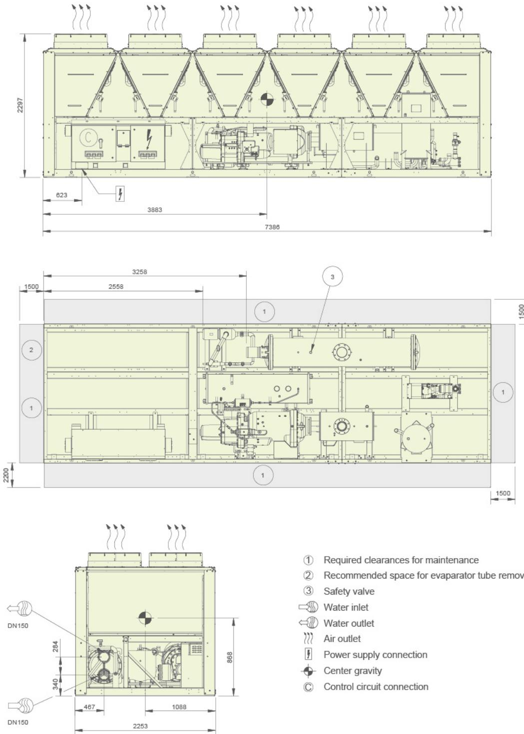
Notes: Single power connection point, and arrive from the bottom. Reserve 120mm height space below the unit for power supply connection (unit aerial installation or cable slot arrangement in unit base)
