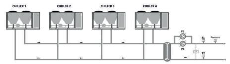
Water-cooled chillers/heat pumps with dedicated dry-coolers, and secondary pumps(1)
