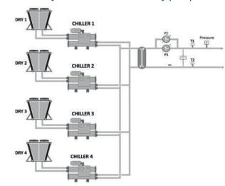
Water-cooled chillers/heat pumps with mutualized dry-coolers, and secondary pumps(2)
